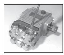
Carefully slide the valve casing (26) out over the plumers.
