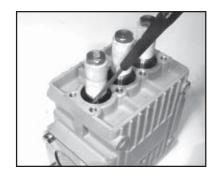
9. If the crankrase oil seals (19) are to be replaced, they can be removed by prying loose with a flat screwdriver. Take care not to make contact with the plunger.
