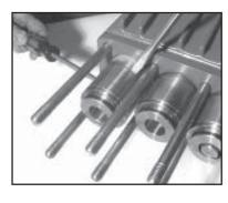
7) Remove the seal sleeve (35) from the manifold and /or crankcase.
