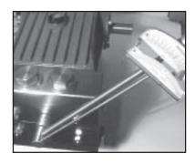
14) Place entire manifold/seal sleeve assembly over the studs and push firmly until seated against the crank-
