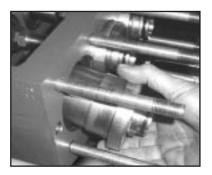
13) Pull seal sleeves (38) and plungers (36) out of their fittings in the crankcase (1) using ring groove as a guide.
