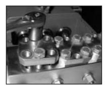
Take plugs (58) out of valve casing (50) by tightening screws (58C) against valve casing with two screws.
