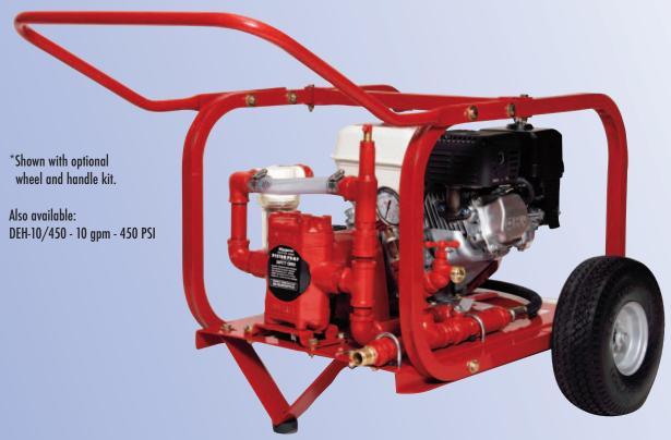
he DE-3C is a mid volume. medium pressure hydrostatic pump. Designed for testing lines up to 16 inches in diameter. This unit is dependable and simple to run. The pulsation damper hose and liquid-filled stainless steel gauge reduce liability and maintenance costs. while providing the user with precise and accurate readings. The positive displacement twin piston pump, is
