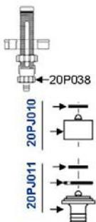
**!** If you experience difficulty removing the upper check valve assembly (20PJ010), try pushing it out with a long screwdriver or similar tool.
