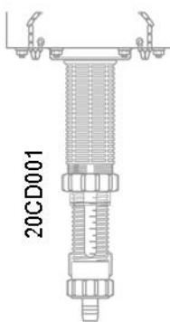
**!** Test the fit on your hose to make sure that there is no air intake during suction. If the hose does not fit tightly, cut a quarter inch off before reattaching.
