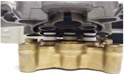
7) Grooved Ring (HP seal, water seal) grooved side down, smooth side up
