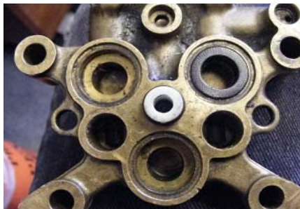
8) Valve & Grooved Ring in place
