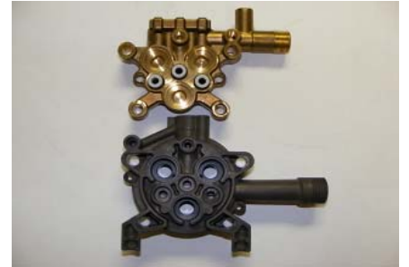
9) Cylinder Head w/valves installed w/Piston Guidance
