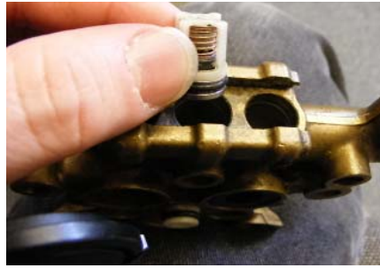
2) Place valve w/1 o-ring in brass cylinder head body, cap/o-ring end in first
