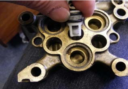
4) Place valve w/2 o-rings in brass cylinder head body, cage end down
