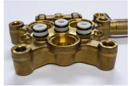
6) All 3 valves installed
